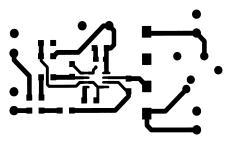
Recommended SOP PC Board Layout: Top Layer
