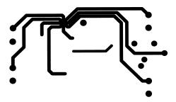
Recommended SOP PC Board Layout: Bottom Layer
